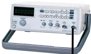
Function generator for measurements in AC experiments RC, RL, RLC circuits
